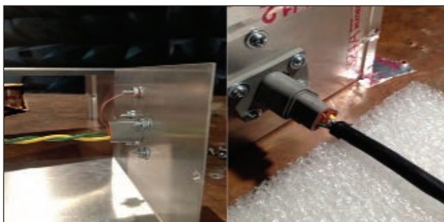
▲ Fig. 12 The experimental setup showing the pigtail connector (left) and the signal cable (right).
