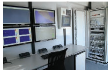
▲ Fig. 4 Complex systems, such as a passive radar system, are designed and deployed with NI LabVIEW software and NI PXI hardware embedded in the final system.
